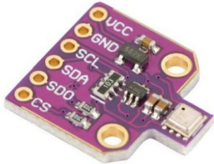
Figure 2. sensor BME680 (source: www.nusabot.id.com )
